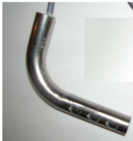
Macro-cell sensor set: 3 sensors placed in a distance of 2 cm from each other with a surface of 1 cm 2 .
