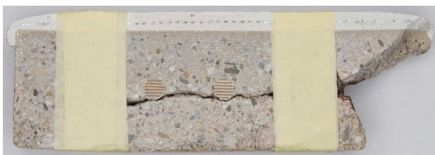
Fig. 2b. EZ-anode/mortar reference probe, stored for 2,5 years under the identical conditions as the galvanic active probe, cut broadside for LIBS measurements
