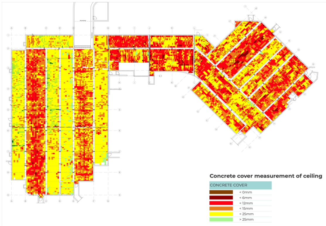
Fig. 23. Cover Measurement Plan - Ceiling Underside
