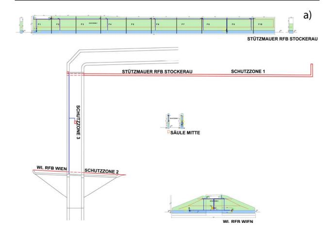
Figure 5: Schematic representation of the CP protection zones & anode system: B2134, sustaining wall – zone 1, bridge column – zone 3, abutment – zone 2.
