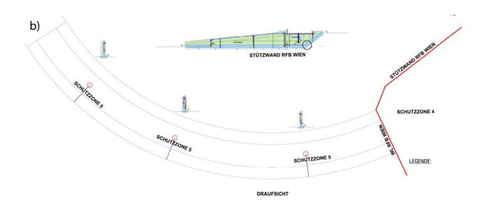
Figure 6: Schematic representation of the CP protection zones & anode systems: B2136, abutment and sustaining wall – zone 4, three bridge columns – zone 5.
