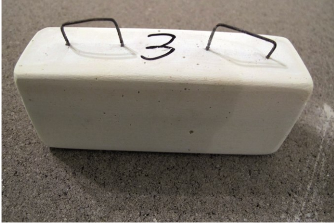
Figure 2: Sika® FerroGard® ICM discrete galvanic zinc anode (SFG-anode) for the prevention of the formation of incipient anodes induced by patch repairs.
