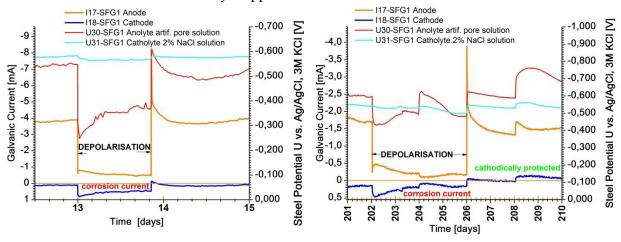
Figure 5: Current and steel potentials during depolarization measurement of a Sika® FerroGard® ICM discrete galvanic zinc anode (SFG-anode) in artificial pore solution two weeks after start up (left) and after 7 month of operation (right)
